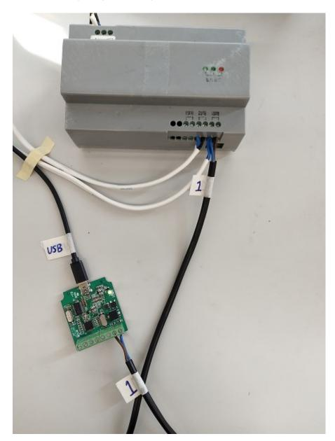
Set the dialer 1 from the back of the OS, 1  $\underline{\text{on}}$  2  $\underline{\text{off}}$  , then power up the device.
